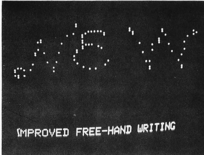
Photo 7: Using the improved circuit of figure 3 reduces much of the over-writing of multiple dots which occurred using the original circuit of figure 1. This is an enhance mode picture.
