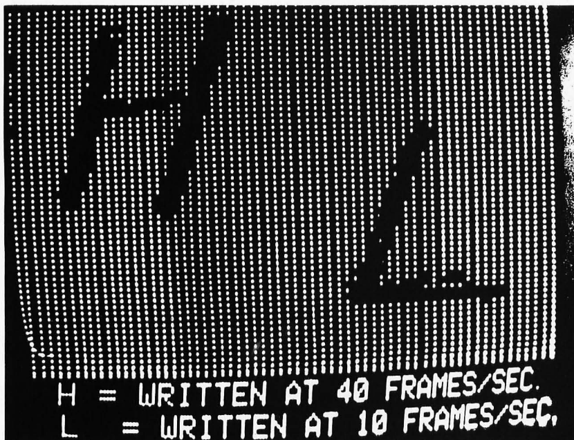
Photo 2: The light pen can be used in an "erase" mode by filling the screen with "on" dots then selectively removing dots with the light pen. The titles added to this picture (and all the pictures in this article) were created with a separate character generator which is not described.
